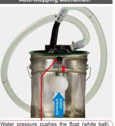
Water pressure pushes the float (white ball) upward and the black part seals the upper suction port.
